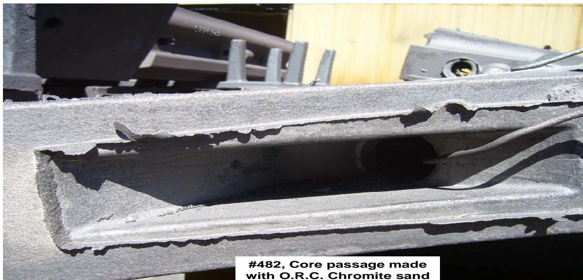
Figure 4. Photograph of casting.
