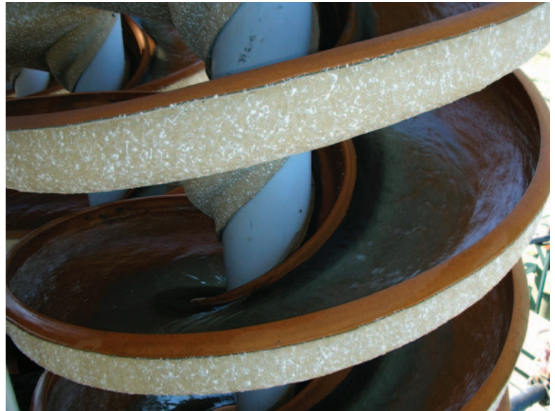
Typical spiral cross section.
