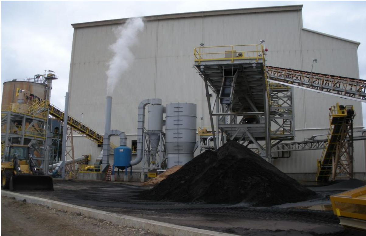
Fig 3: Heavy mineral concentrate in the foreground and fluid bed dryer and dry mill in the background, June 2011.
